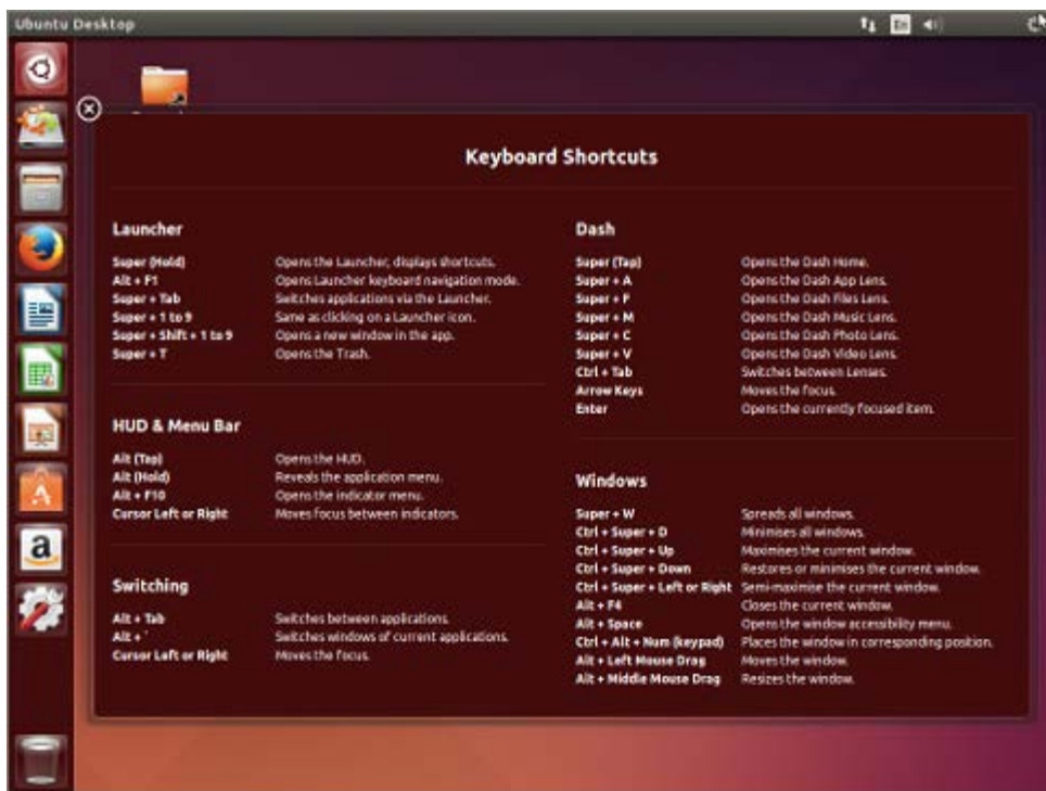
Figure 5. Holding down the Unity Super key displays a list of common keyboard shortcuts.
